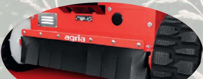
Protection against thrown objects: Safety flaps tested by DLG
