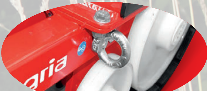
Safe loading with eye bolts
