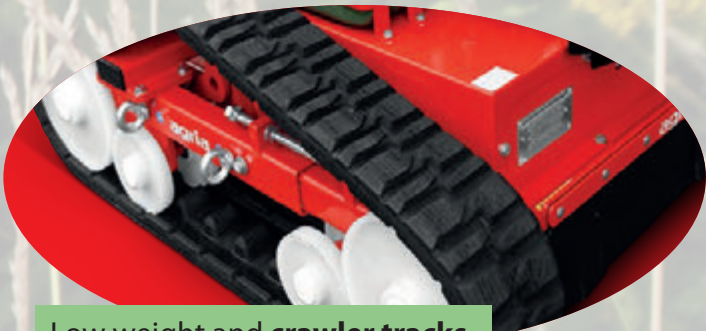
Low weight and crawler tracks to protect the soil
